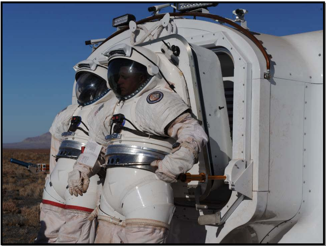
Fig. 1. Prototype LER suit ports being developed by NASA. The LER rover concept relies heavily on safe and efficient suit purge and prebreathe protocols to minimize gas losses and enable rapid vehicle egress.
